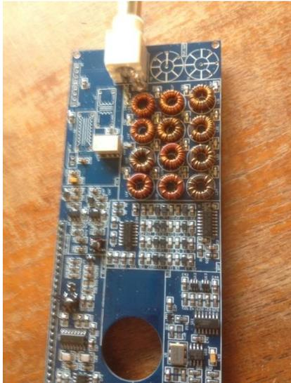
3. I then added the two 10:1 swr toroids. I checked with Chris and he recommended 10 turns on each toroid and a single loop to complete the transformer.
