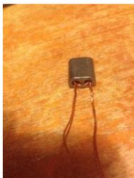
8. Winding the 3:2 transformer. This was simple. Two turns from one end, three turns from the other. I marked the two turn end so it could be positioned accurately on the pcb. See below:
