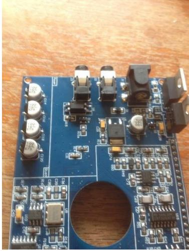
5. I then fitted the two FETs to the three left hand pcb holes. This left one empty hole to the right of each device – see below. Position carefully as far inward as possible as the heatsink may not fit the case later. In my case I had to bend the FET legs slightly to enable an accurate fit once the case was assembled.
