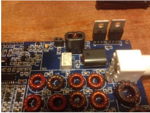
9. Fitting the heatsink. This is straightforward. However I needed to attach the FETs with nuts and bolts as the supplied screws did not tighten correctly. Not an issue. It is worth spending some time to make sure the heatsink is level so that it fits the case nicely later on.
